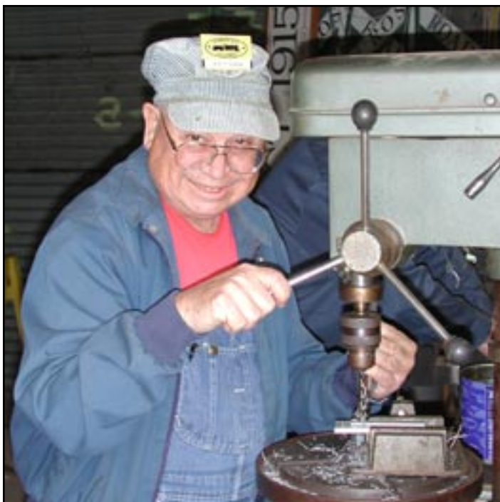
Jack Friedman with a steady hand drilling track bars used to join the rail together.
