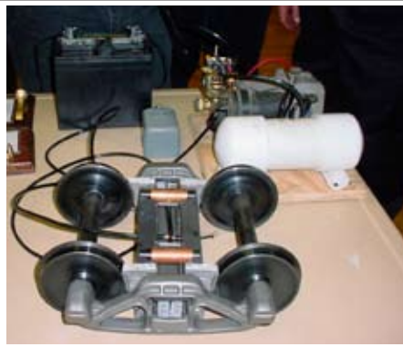
Milon Thorley showed a working brake system (Tom Bee's) that uses an air pump from a GM auto where the pump was for air load levelers.
