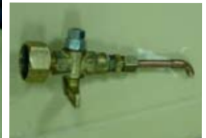
Ross Crawford made this tool to clean the inside of your engine by inserting it through a fitting which then allows you to rotate the nozzle.
