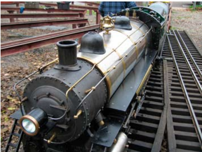
First the head lamp wiring was move and given its own conduit so the hand rail could be redone allowing it to loop the front of the engine.
