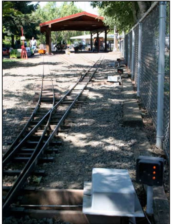
WCRR Track view to station, notice the electric switch machines and indicator lights showing direction of switches.
