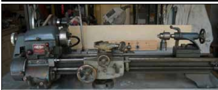
Wards (Logan) Power-Kraft Model 25TLC-2136 Back Geared Screw Cutting Lathe with Quick-change Gear Box 10" Swing - 1-1/2"-8 #3 MT Spindle Bore 50" Bed Length - 31" Between Centers Spindle Bore 25/32 Includes: 3-Jaw & 4-Jaw Chucks, Jacob's Chucks for Headstock & Tailstock, Collet Set, 6" Face Plate, 110 Volt Flat belt drive $1000 Contact: Mike Dreiling 916-729-2200 or 916-201-0888(cell) email mdreiling@macnexus.org
