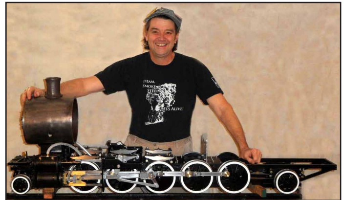
Dave August shows his 2-10-2T chassis completed and running on air.
