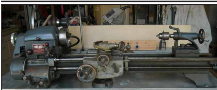
Wards (Logan) Power-Kraft Model 25TLC-2136 Back Geared Screw Cutting Lathe with Quick-change Gear Box 10" Swing - 1-1/2"-8 #3 MT Spindle Bore 50" Bed Length - 31" Between Centers Spindle Bore 25/32 Includes: 3-Jaw & 4-Jaw Chucks, Jacob's Chucks for Headstock & Tailstock, Collet Set, 6" Face Plate, 110 Volt Flat belt drive $1000 Contact: Mike Dreiling 916-729-2200 or 916-201-0888(cell) email mdreiling@macnexus.org
