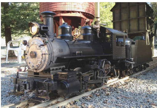
Freelance 7.5" Gauge 0-4-0, 7.5" Gauge, 1.5" Scale, Oil Fired, 2" Winton Cylinders
