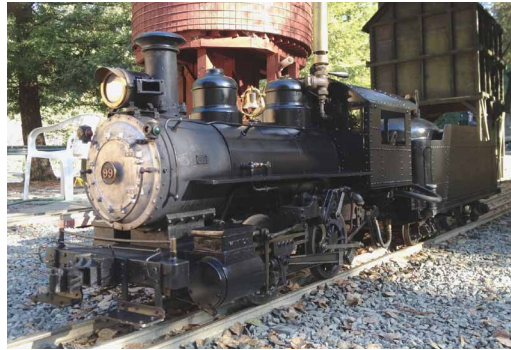
Freelance 7.5" Gauge 0-4-0, 7.5" Gauge, 1.5" Scale, Oil Fired, 2" Winton Cylinders
