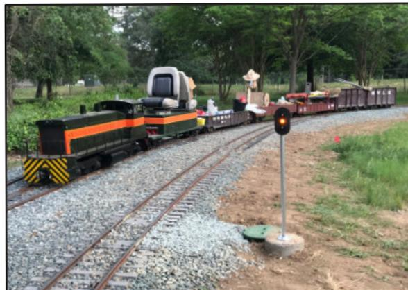
The signal system is in phase one. This shows that the inside loop is occupied and will give a "clear" to the train in the loop when there is not traffic on the main line from the box car yard or the line out the north gate. If there is a train in the loop and traffic is approaching the crossing they will get a stop until the train clears the loop.
