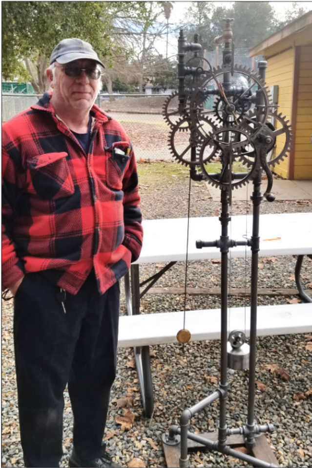
John shows his home made clock, he designed a unique gear set. Clock will run 36 hours per wind.
