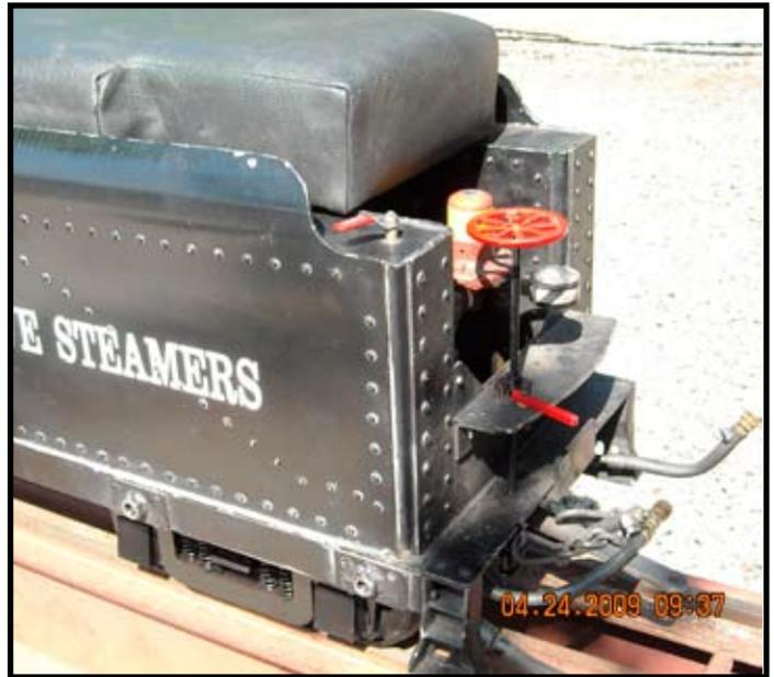
New Brakes on tender controlled by engine or hand wheel
