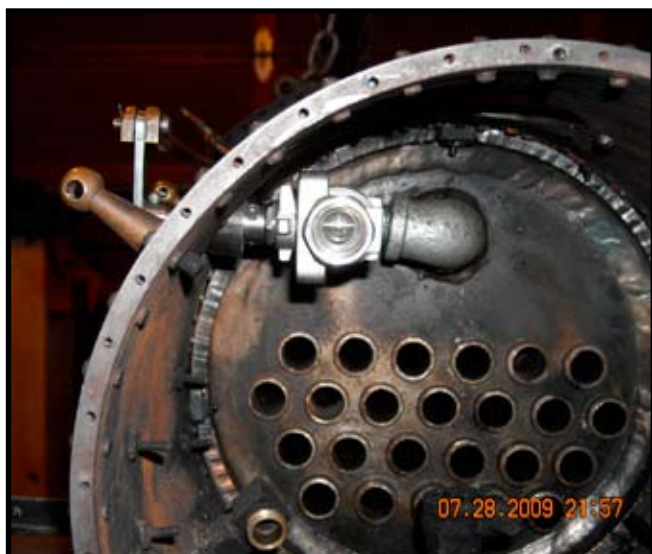
#1973 Smoke Box showing throttle valve
