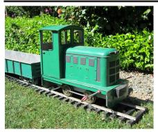
1" scale, 4.75" gauge train consisting of : Maxitrack 0-4-0 side rod diesel (new transistor throttle, professionally rebuilt motor, battery) , 2- Scale RR Supply gondolas (50" long with SKF sprung, roller bearing trucks, 1 painted, 1 aluminum)
