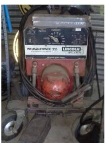
Engine driven Welder Generator. Lincoln Welder 225 amp. With cables.
