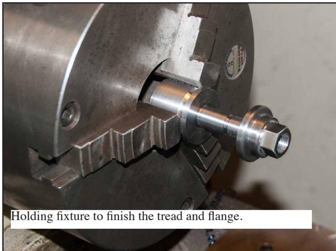
Holding fixture to finish the tread and flange.
