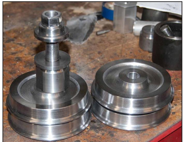
Finished wheels waiting for axles. The three flats on the holding fixture allow the fixture to be indexed to the number 1 chuck jaw, and the flange holds it the same dimension from the face of the jaws in case the fixture needs to be removed and then re-used on the same project.
