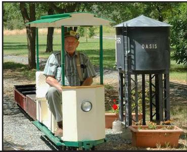
1 1/2 scale, 7 1/2 " gauge 4 wheel Diesel locomotive with 5hp Briggs & Stratton engine. Hydraulic powered. Easy to run and maintain. Flat car support car included . Has Mountain Car trucks and couplers.
