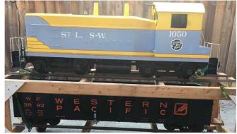
Features included: Rigged to run cab forward, may be changed to hood forward. Head lights Horn Reliable Honda motor, very fuel efficient. Upgraded Eaton hydrostatic transmission. Prototypical correct automotive paint, applied by body shop. Fresh Miracle vinyl graphics. Marine quality wiring Brake system compressor system using premium Gast compressor. Air brakes installed in engineers car. Battery charging by magneto and installed charging port Trickle charger included. Safety cables.
