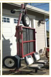
drive has been installed as well as a pressure driven air brake system using a GAST 12 volt compressor.
