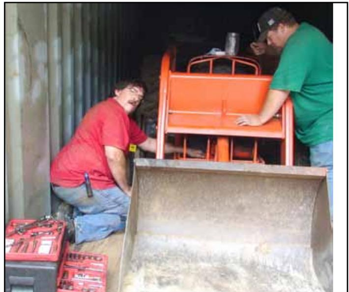
Ben Klienwacher and Richard Lutrel replacing coupler so we can use the tractor to move gravel once again.
